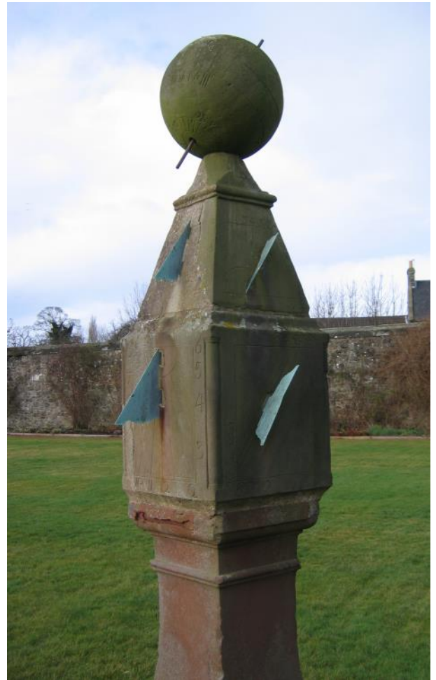
Fig. 8. The multi-faceted dial showing the reclining faces.
