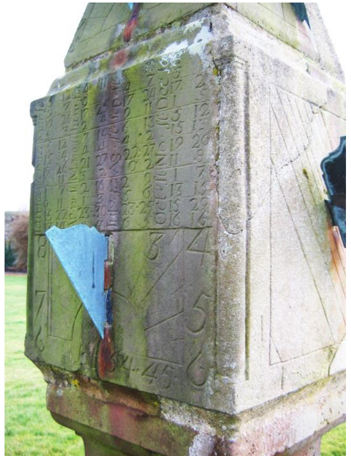
Fig. 9. The north face of the multi-faceted dial showing the latitude and the non-intuitive EoT table
